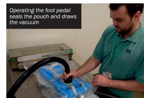
Operating the foot pedal seals the pouch and draws the vacuum
