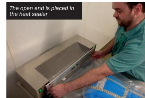
The open end is placed in the heat sealer
