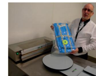
pouch is slid over two metal rods which open the pouch up as it is pulled forward so that it easily covers the wrapped set. The turntable and set is then swung around, enabling the open end of the pouch to be placed in the heat sealer. The nozzle from the vacuum is then attached to the pouch’s vacuum valve.
